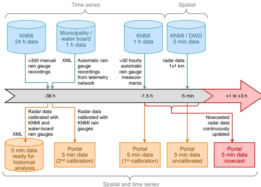
**Fig. 4** Process-flow diagram for calibration of radar data to create the best composition of information in real-time and post processing of data to generate up-to-date and calibrated spatial and time series.
